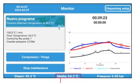
Temperature recorded by the first flexible probe.
