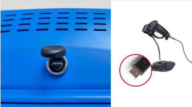
1. Connect the barcode scanner to the USB port located at the top rear of the autoclave.
